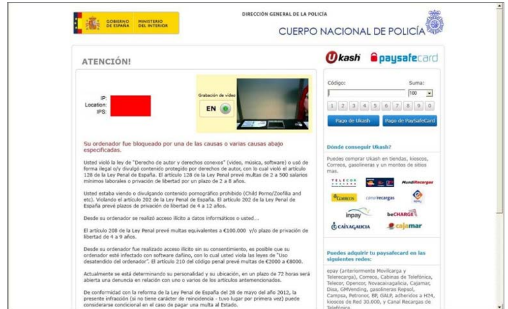
FIG.02. NEW WARNING USED BY THE POLICE VIRUS, SHOWING THE IMAGES CAPTURED BY THE COMPUTER'S WEBCAM.
